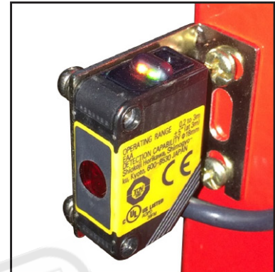
Power on & aligned
